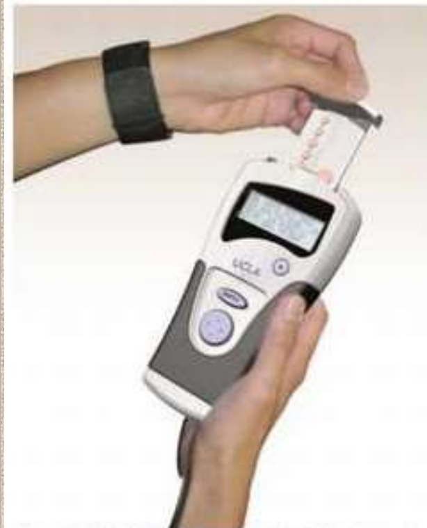
Figure 4. Oral Fluid NanoSensor Test, a handheld, automated, easy-to-use integrated system that will enable simultaneous and rapid detection of multiple salivary protein and nucleic acid targets.
